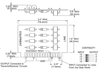
NOTE: I/O contacts spaced at 0.156" (3.96 mm) centers
